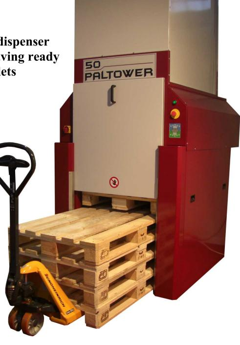
By using a hand pallet truck 1 to 5 pallets can be simultaneously loaded and unloaded at ground level.
